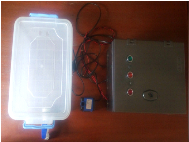
Appendix II: Control System Panel, Centrifugal Submersible Pump and Water Tank
