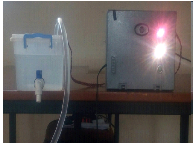
Appendix V: Yellow LED- Level 2 Reached Indicating the Tank is Half Filled
