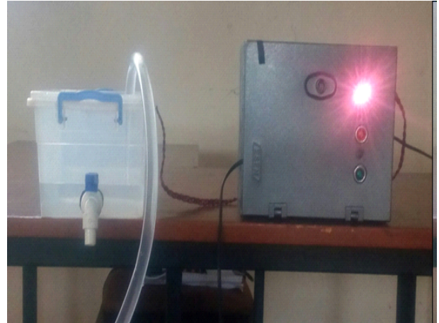
Appendix IV: Red LED- Level 1 Reached Indicating the Tank is slightly Filled
